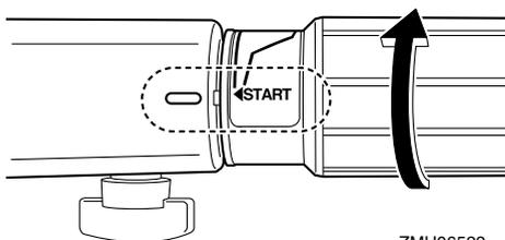
4. Pull the manual starter handle slowly until you feel resistance. Then give a strong pull straight out to crank and start the engine. Repeat if necessary.
