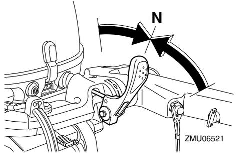
2. Place the tilt lock lever in the release/up position.
