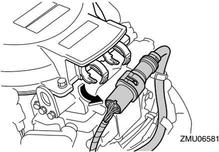
3. Remove the flywheel magnet cover after removing the bolt(s).
