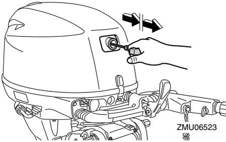
6. After the engine starts, slowly return the manual starter handle to its original position before releasing it.
