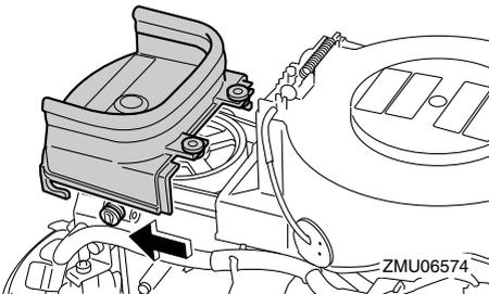
2. Remove the grommet and disconnect the start-in-gear protection cable from
