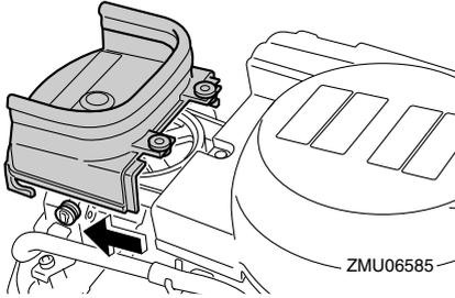
2. Pull off the 10-pin connector from the clamp and remove the flywheel magnet cover (if equipped).
