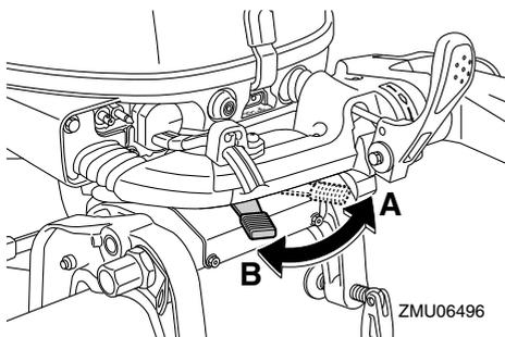
If the resistance does not increase even when the lever is turned to the port side “A”, make sure that the nut is tightened to the
