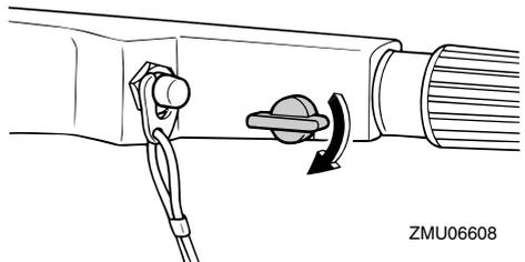
5. Pull the manual starter handle slowly until you feel resistance. Then give a strong pull straight out to crank and start the engine. Repeat if necessary.
