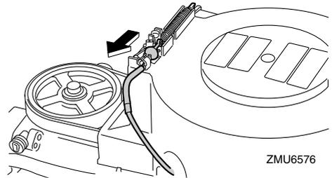
3. Remove the manual starter after removing the bolt(s).
