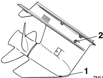
1. Gear oil drain screw
